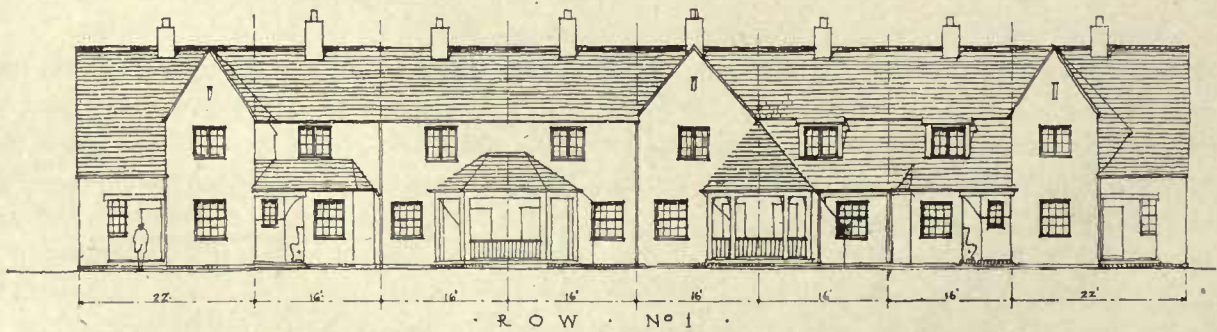
Typical Elevations of Street Fronts and House Rows. Hilton Village.—Francis Y. Joannes, Architect.
