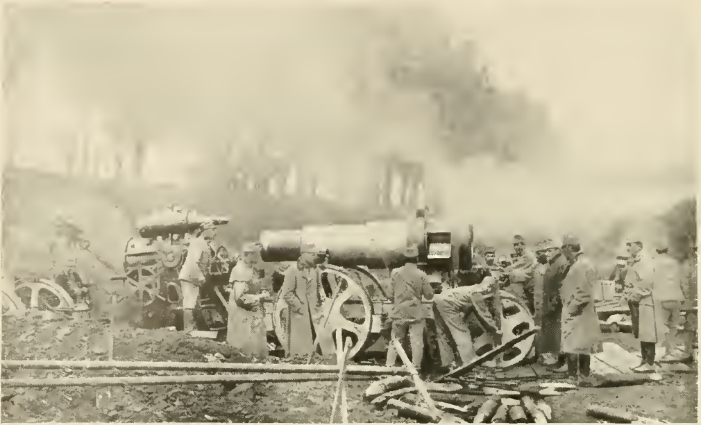
Austrian Artillerymen and Mechanics Assembling a Giant 30.5 Cm. Siege Gun for the Second Bombardment of Przemysl, June, 1915.
