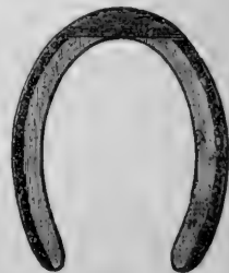
Fig. 9. Shoe for Raised Coronet, showing where to nail.
