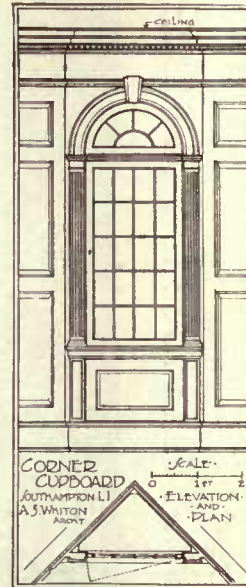
Figure VI—In building a Colonial corner cupboard it is necessary to reproduce as closely as possible the panelling of the room. A working drawing is shown below
