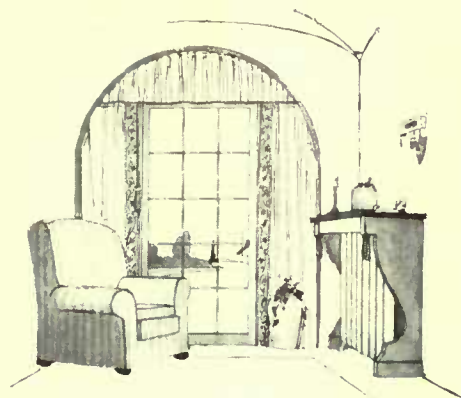
In an enclosed porch a shelf can be built above the radiators, supported by side brackets. The top may be marbleized
