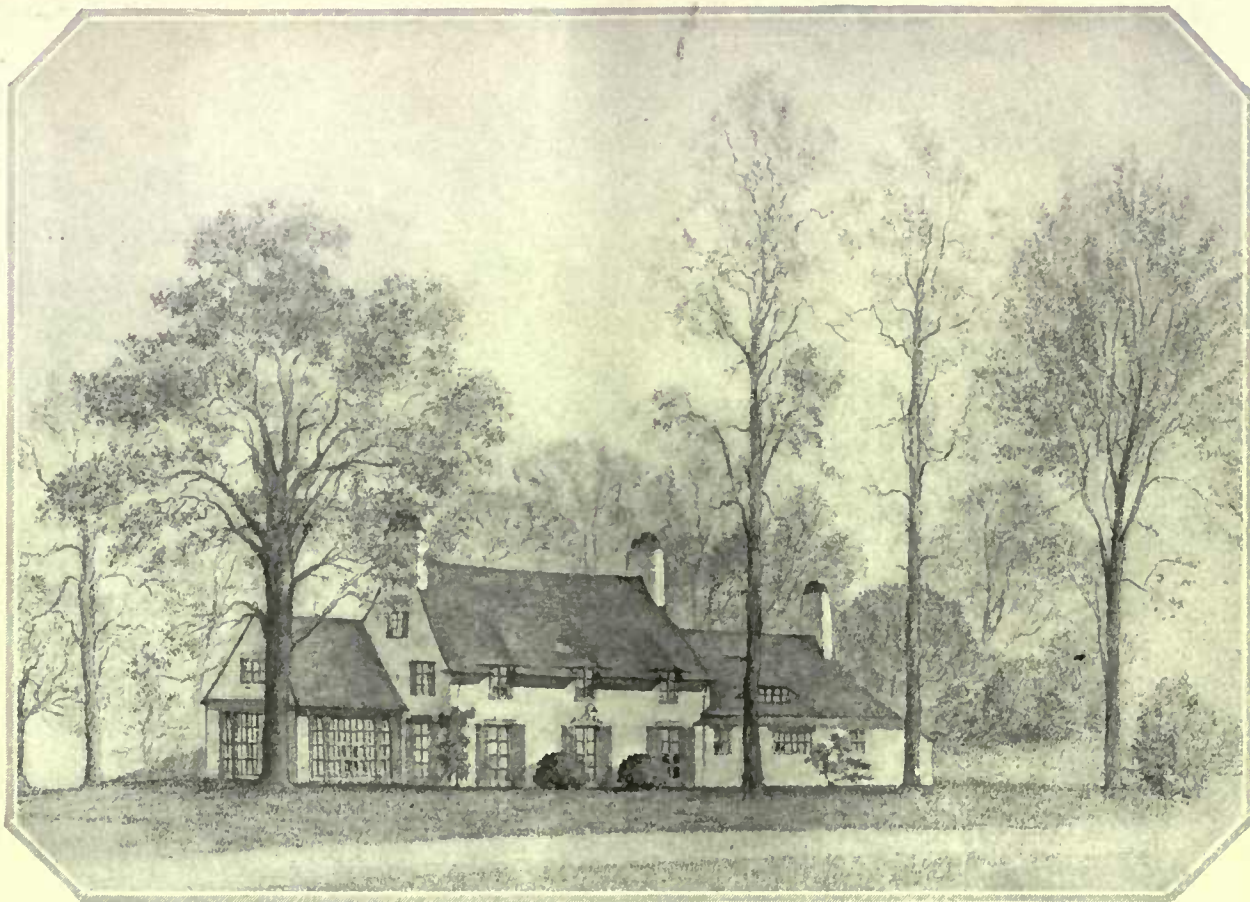
The preliminary sketch is really a picture of the finished house, drawn in perspective and usually colored. It shows the house with its surrounding planting well established, and gives a definite idea of what the house is to look like. H. T. Lindeberg, architect
