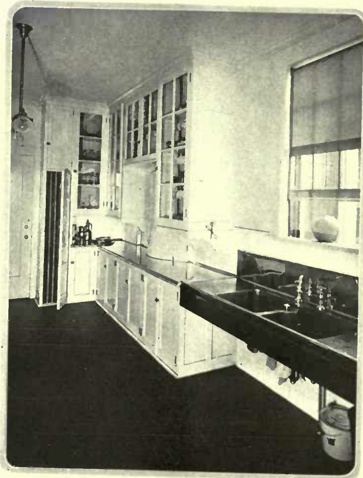
In designing a pantry, space must be afforded for everything that is to be put away, as, for example, the rack for the table leaves in this pantry
