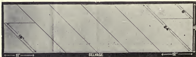
FIG. 23.—Estimating the amount of material required for bias trimming when part or all of corner can be utilized.
