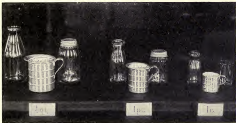
FIG. 24.—Measures commonly used in the household. Metal measures are usually the most accurate and convenient.
