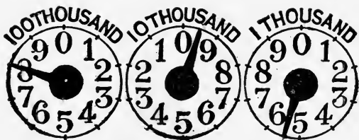
FIG. 11.—Gas meter—index reads 79,500 cubic feet.
