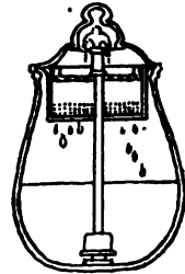
FIG. 173. — Cross section of a coffee percolator.
