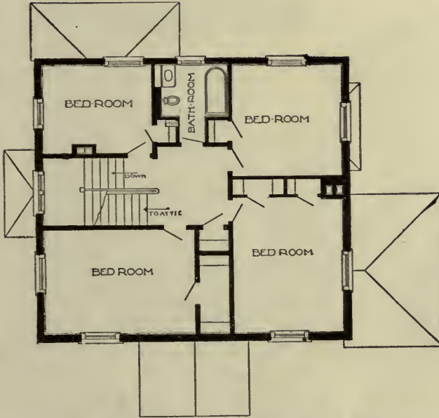
PLAN No. 9. Second Floor. Good Closet Room. Clothes Chute in the Bath Room. Scale \frac{1}{8} inch=1 foot. Messrs. White and Temple, Architects.
