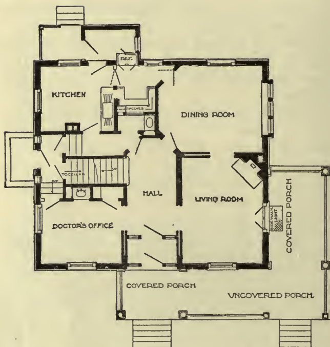
PLAN No. 9. An Excellent Arrangement of Rooms in a House Nearly Square in Plan. Compact Stairway. Side Entrance for Doctor's Patients. Convenient Kitchen, Pantry and Refrigerator. Note Side-walk Light in the Covered Porch to Admit Light to the Cellar.
