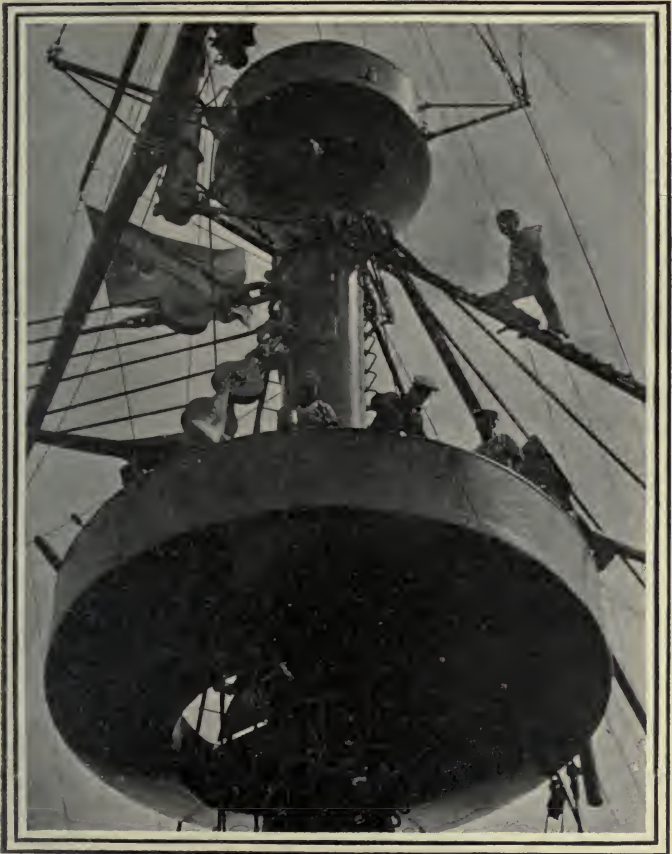
The fighting-top of a battleship. The men reach the platform through an aperture so small that very stout men cannot pass through it.
