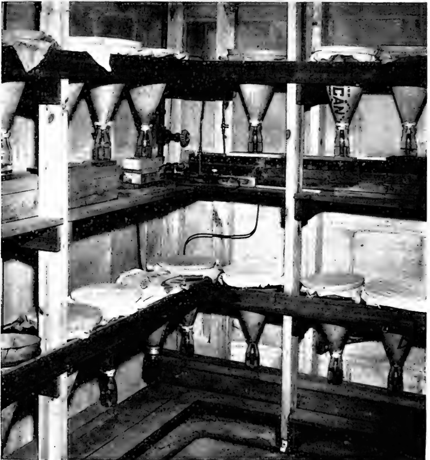
Fig. 8.—Berlese funnel in position on rack. Each funnel rests inside a double ring of copper tubing (visible at extreme lower left), through which live steam flows. The steam produces heat that dries out the sample of leaf mold in the funnel and drives animals into a bottle of preservative below. Cotton or a small rag is tamped between the end of the funnel and the mouth of the bottle to prevent escape of specimens.
