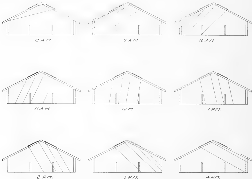
Fig. 1—Relative position of sunlight at different hours March 10, in Iowa Sunlit Hog House for Central Iowa, 42° N. Latitude—Marshalltown, Ames and Carroll, Iowa.
