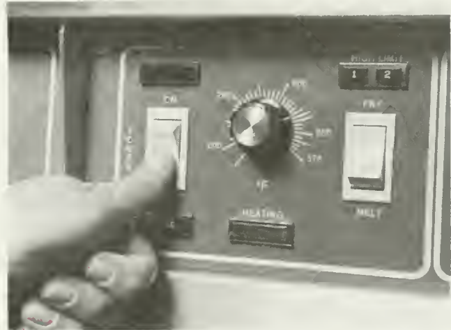
Control of new high-efficiency fryer, set at economical 330° level.
