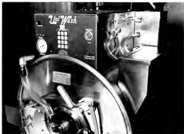
Microcomputer on newer model clothes washing machine permits precise control of water temperatures, cycles.
