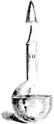
Bulb with capillary orifice for testing small quantities of matter. p. 200.
