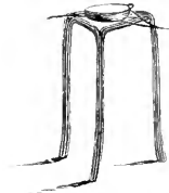
Tripled wire stand for holding platinum. p. 43.
