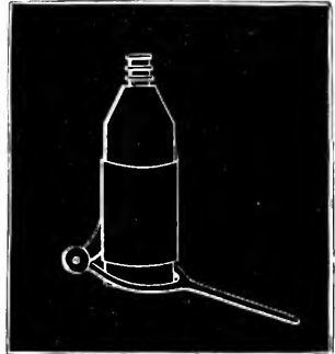
Achromatic condenser mounted with a lever. Landis. p. 11.
