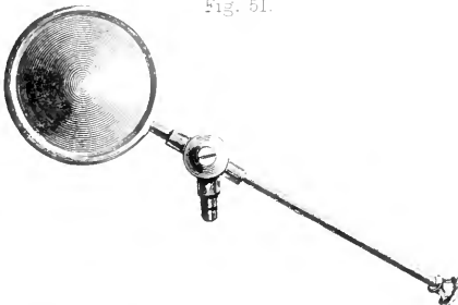
Coll's cylindrical condenser for students' microscope. p. 21.
