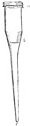
Pipette serving as the stopper to the bottle. a, rubber and India rubber by pressure which fluid may be expressed from the tube b around to fit the neck of the bottle. c, the orifice. p. 210.
