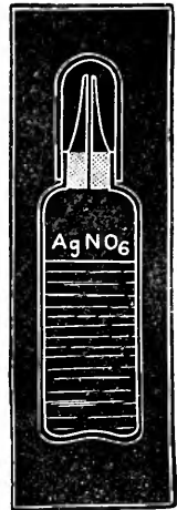
Small test bottle, with capillary orifice. p. 200.
