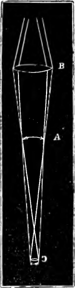
Diagram of compound microscope. A point where the object is brought to a focus in the objective glass. C the image formed at this point is magnified again by the eyepiece B. p. 4.
