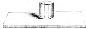
Cell for examining solutions by the spectrum microscope. Half the real size. p. 219.
