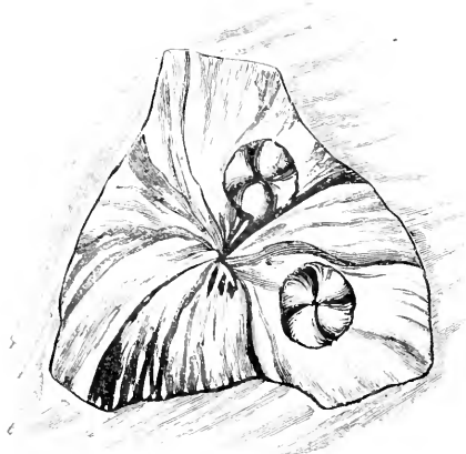
Copper crystalline plate, crystallized at 100°.
