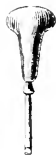
Large bradawl, for scraping away superfluous marine glue in making cells. p. 62.
