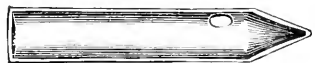
Glass slide for examining solutions by the spectrum microscope. Half the real size. p. 220.
