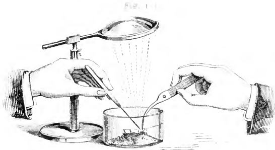
Fig. 141. Instrument for mixing minute doses of salts under water. p. 74
