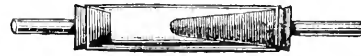
FIG. 66.—Marey's sphygmoscope, which acts as an elastic manometer in connection with a tambour. It consists of a cylindrical glass tube, closed at both ends by rubber stoppers with a hole through the centre of which come two glass tubes. An elastic cap is slipped over the right-hand stopper, filled with an anticoagulant solution, and connected with a blood-vessel. The cap reacts to each rise and fall of pressure, by expanding or contracting. The tube on the left-hand side conveys these movements to the tambour.
