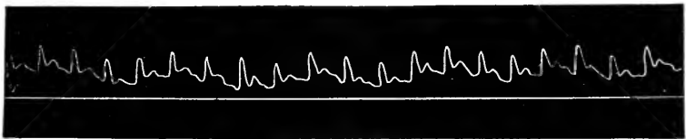
FIG. 117.—V, Plethysmogram of hand taken with apparatus of Fig. 115, the oscillations of the column of fluid being suppressed by the bulb interposed between the exploring apparatus and the recording tambour. (Fr.-Franck.)
