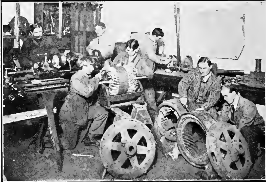
Students winding a 10-h-p-Induction Motor in the Electrical Laboratory
