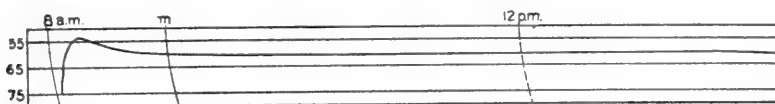
FIG. 16.—Variations in volume of double trio of sections of agar and peptone which had reached full hydration in distilled water and were then immersed in calcium chloride, 2M.
