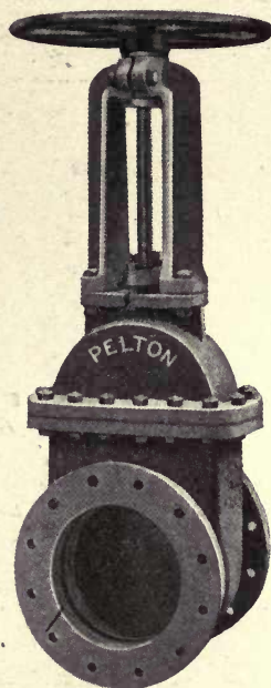
Fig. 111. Straightway Valve of Single-Disc Type, with Rising Spindle, Intended for Pressure on One Side Only. Disc rises clear of opening, giving a perfectly free way for the water. Seats are of bronze, to be replaced when worn.
