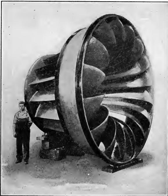
FIG. 172.—High-speed turbine runner. D = 102'' ; h = 76' ; N = 120 ; Hp = 20,000 .
