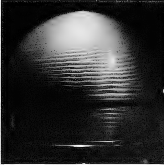
Fig. 6 The vortex axes become wavy for very large Reynolds number. s = 2 mm, Re = 16,800 , Ta = 68.8
