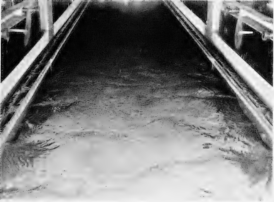
Fig. 15. Sample view of wind-waves obtained for a 4 m/s velocity and a 4 m fetch.
