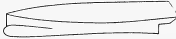
A Cusped Cosine - Parabolic with Bow Bulb and Transom Stern ( x \neq 0 )
