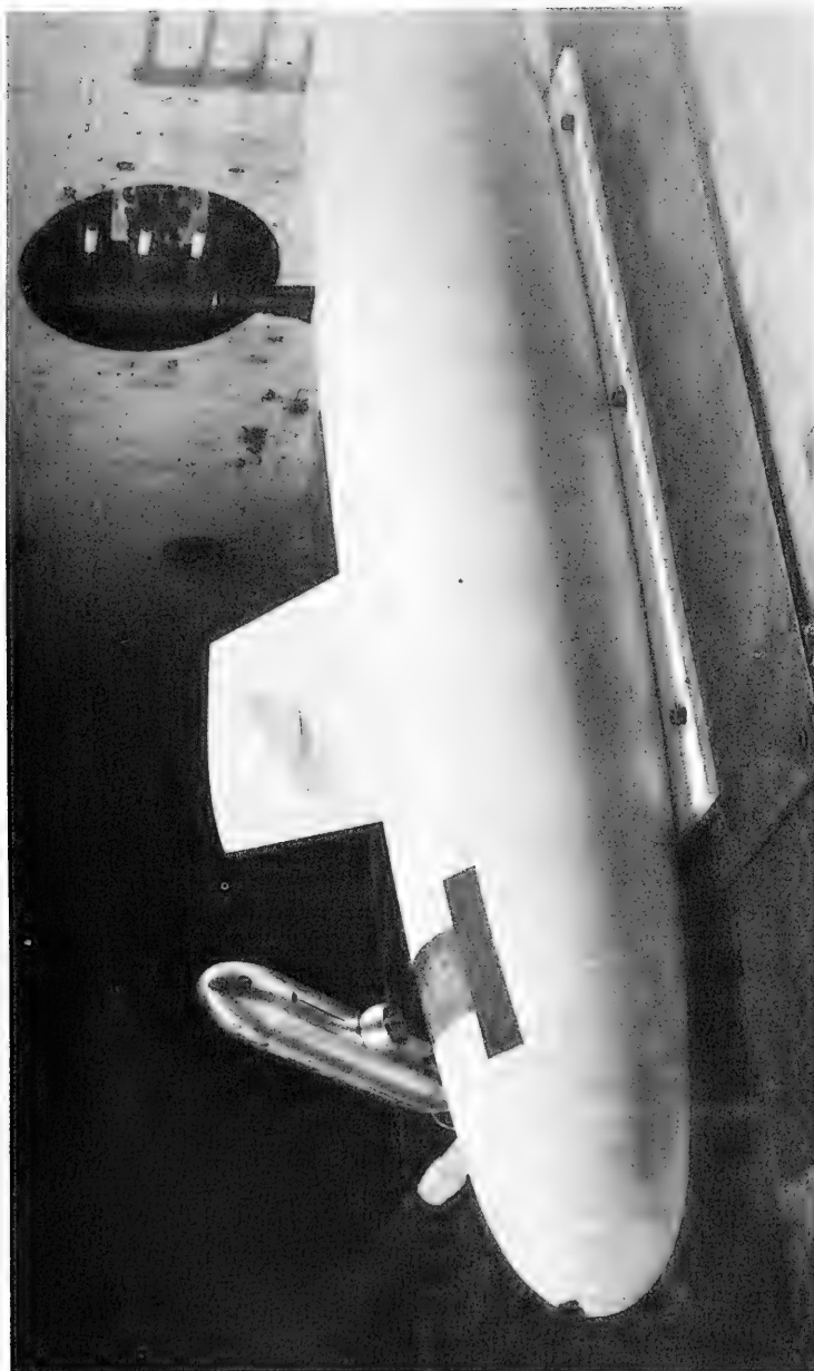
Fig. 15. Model Installation-Mating on the Forward Hatch with a Submarine Heading of 90 Degrees
