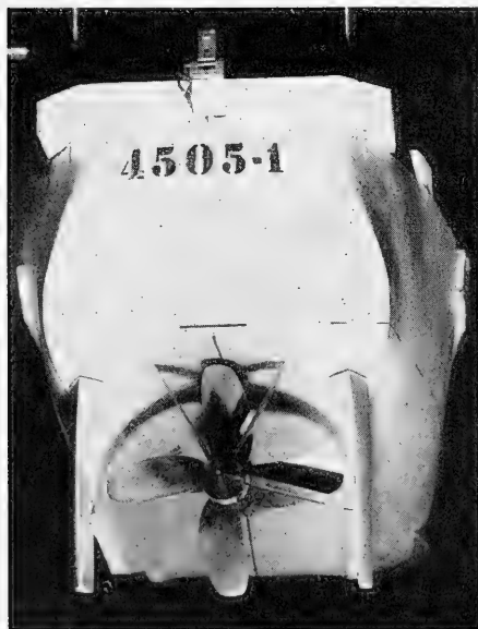
FIG. 67.N VIEW FROM AFT OF ARCH-STERN ASSEMBLY ON ABC SHIP MODEL
