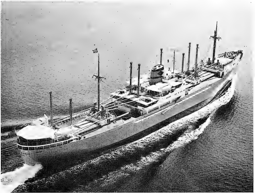
FIG. 49.E AERIAL VIEW OF A SHIP, SHOWING RELATIVELY SHARP TRANSITION BETWEEN HOLLOW ENTRANCE WATERLINE AND PARALLEL WATERLINE AMIDSHIPS
