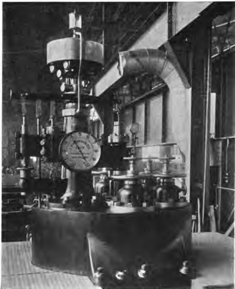
FIG. 139.—Large Capacity Hydraulic Governor. (Built by I. P. Morris Company.)
