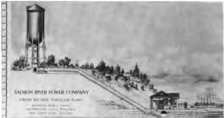
FIG. 69.—Cross-section of Salmon River Power Company's Development.
