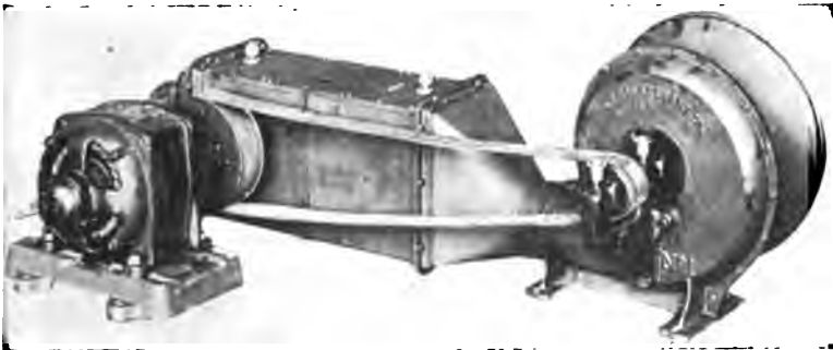
FIG. 282.—Hot-air Drying Outfit for Transformers.
