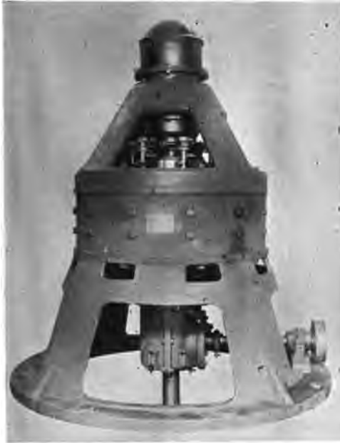
FIG. 210.—Vertical Water-wheel-driven Exciter, Showing Thrust Bearing at Top.
