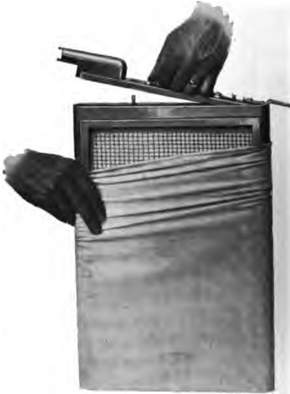
FIG. 203.—Peterson Filtering Unit, Showing Method of Placing Bag Over Frame.
