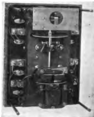
FIG. 322.—Polyphase Induction-type Reverse-power Relay. Cover and Register Removed.
