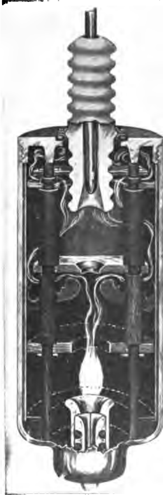
FIG. 309.—Oil Vessel for High-capacity Oil Circuit Breaker Showing Oil Baffle Arrangement and Contacts.
