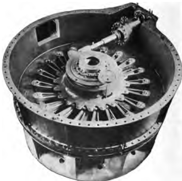
FIG. 128.—Vertical Reaction Turbine, Showing the Gate-operating Mechanism and Speed Ring. (Built by I. P. Morris Company.)
