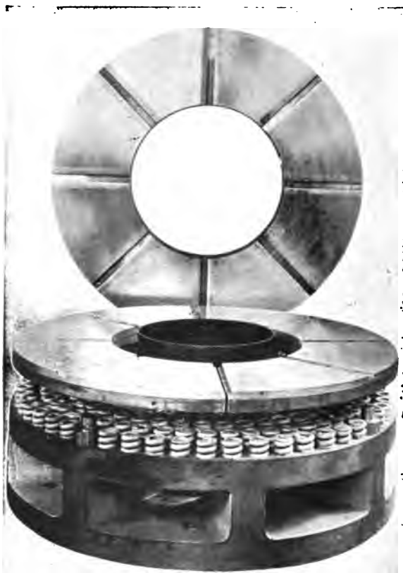
FIG. 198.—Spring-supported Thrust Bearing, Showing Rubbing Surface of Rotating Ring; Stationary Ring with Sawcut is Raised to Show Arrangement of Springs.
