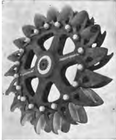
FIG. 133.—Tangential Water Wheel Equipped with Ellipsoidal Interlocking Chain Type Buckets. (Built by Pelton Water Wheel Company.)
