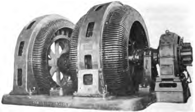
FIG. 209.—3000-K.W. Frequency Changer Set, Showing Mounting of Direct-connected Exciter.
