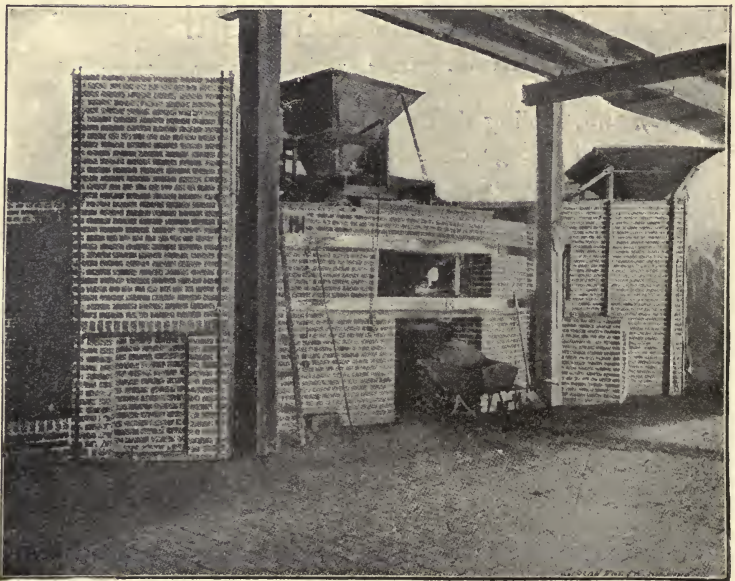
FIG. 111.—FEEDING HOPPER AND DISCHARGE OPENINGS OF PEARCE TURRET FURNACE.
