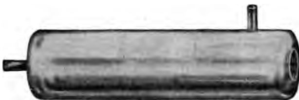
Fig. 130.—Elbrecht's apparatus, representing a metal heating chamber, block tin lined, with opening for electric heating unit and rubber tube connections for intake and outlet of saline solution. (One-third size.)
