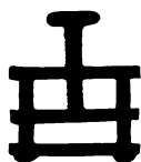
Fig. 134. —Pinch-cock used entirely to close flow or for drop method. (One-half size.)
