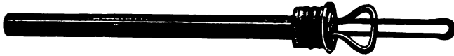
Fig. 132.—Heat unit for alcohol or Bunsen burner flame with regulating piston. For use where electric current is not available. (See Fig. 130.) (One-third size.)
