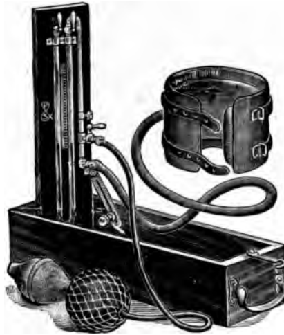
Fig. 5.—Faught's blood-pressure apparatus.
