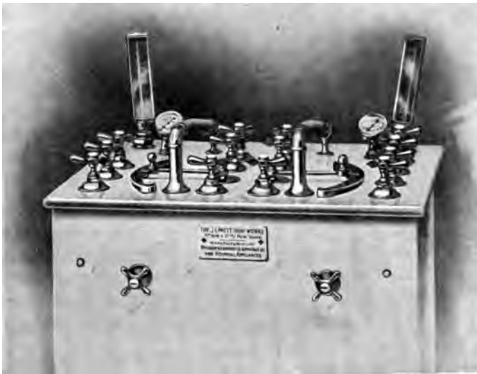
Fig. 78.—Hydriatic control table with polished Italian marble sides and top, fitted with two mixing chambers, each with temperature-regulating valve, pressure-regulating valve, thermometer, gauge and electric alarm for indicating high temperature, two special nozzles, with tips of three different sizes, quick-opening compression valves for the admission of hot, cold, and ice-water to the table, also compression valves for the control of the water to the various fixtures and douches (J. L. Mott Iron Works).
