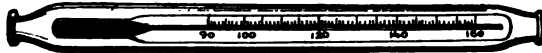
Fig. 139.—Irrigating or infusion thermometer for measuring the temperature of saline solution, or by cutting the rubber tube it can be inserted between the irrigator and the patient by slipping the tube over each end of the glass tube that holds the thermometer.
