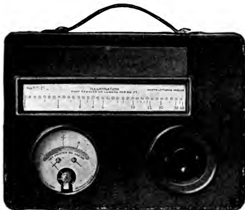
Fig. 52.—A foot candlemeter which is portable and easy to use in measuring light intensities. (Courtesy of the National Lamp Works, Cleveland, Ohio.)
