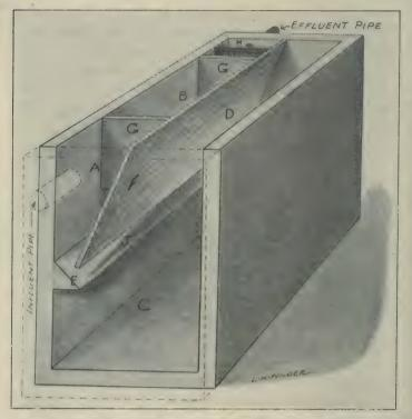
Fig. 40.—Imhoff Tank. The water flows through the upper chambers of the tank A and B, the flow being reduced by the baffles G; the upper chamber is separated from the lower or sludge digestion chamber C, by the partition F; the solids settle out through the slot J, and the gases escape to the right D, being separated from the fresh sewage. (Public Health Bulletin No. 101.)
