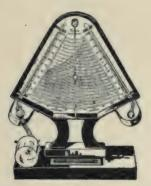
Fig. 51.—Hygrodeik showing the chart from which the condition of the air may be read directly. This is the most satisfactory instrument for telling moisture content quickly. (Courtesy of the Taylor Instrument Companies, Rochester, N. Y.)
