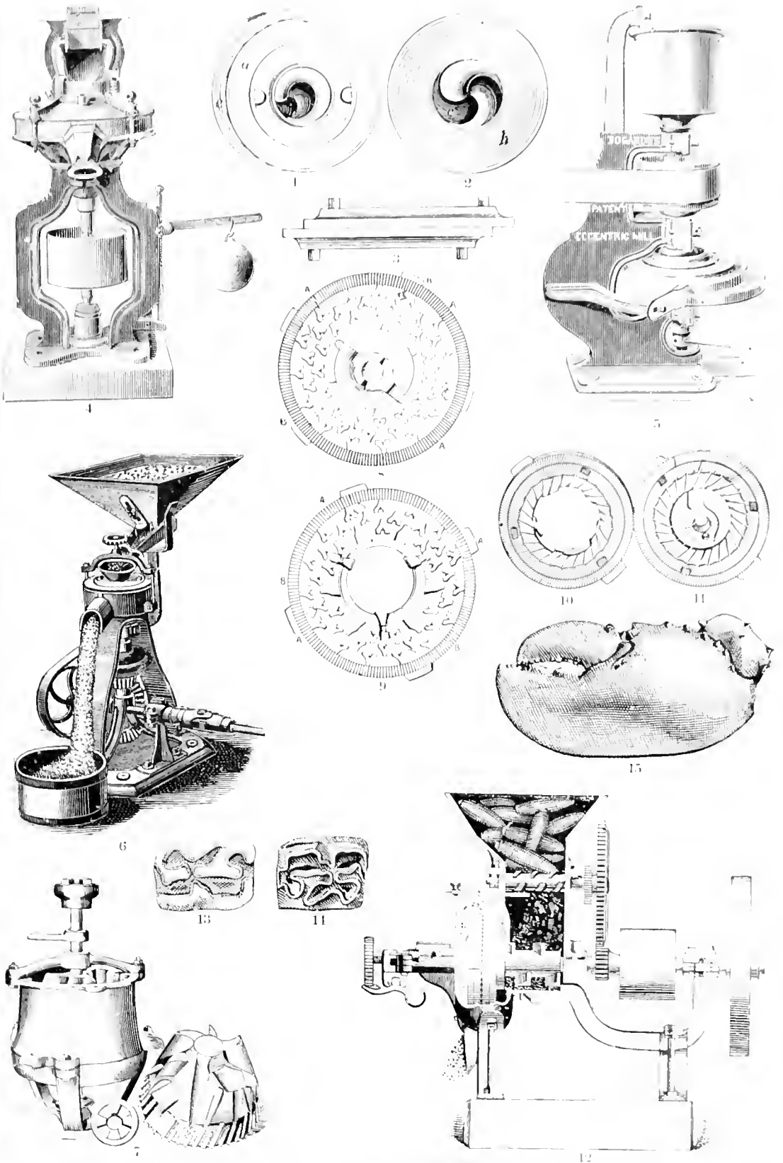
1. Face of grooved plate, 2. Edge view, 3. Plan of superior plates, of the "Bovinus" mill, 4. Elevation of the "eccentric" mill for dry substances, 5. "Eccentric" mill for wet substances, J. S. & C. L. Sisson, Boston, N. Y., 6. Elevation of a corn mill, 7. Corn and cob crusher, 8, 11. Grinding plates, 12. Elevation (partly in section) of the "Scott" mill, 13. Cross section, 14. Crown, of horse teeth, 15. Foster claw.
