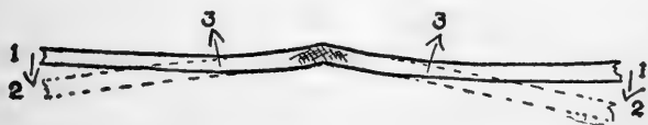
Compound lateral bend (both angular and curved deflections), viewed from rind side of strip
