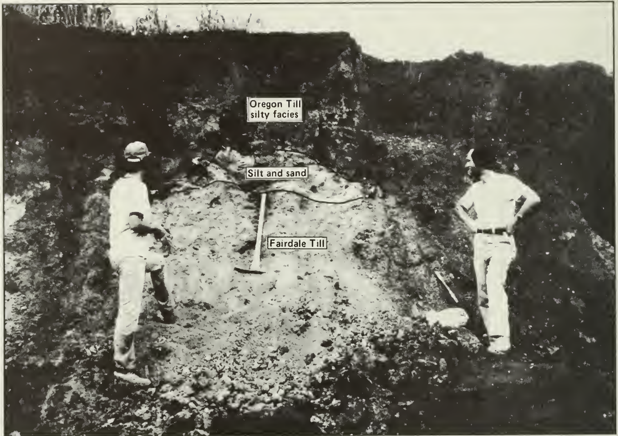
Figure 9-3 Photograph of Profile 2 showing the Oregon Till silty facies above the Fairdale Till.
