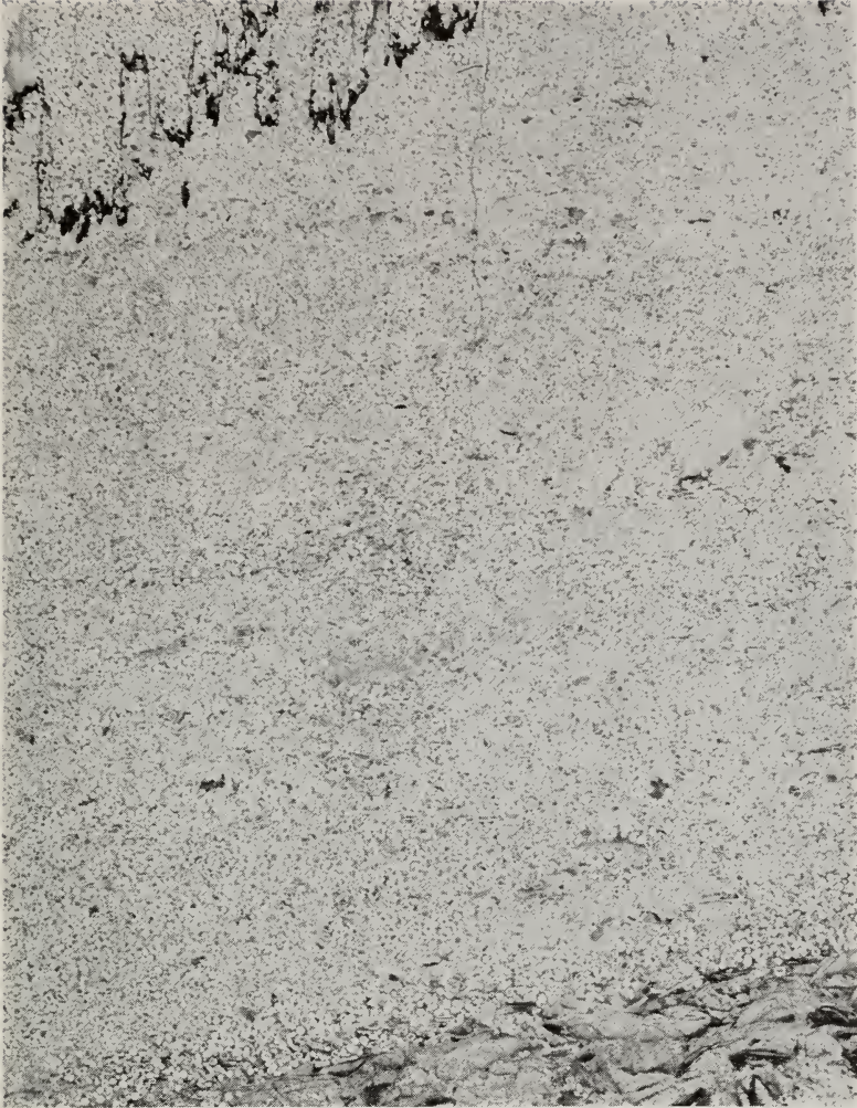
FIG. 11.—Limestone marble from the Ste. Genevieve formation. Cut at right angles to the bedding. Natural size.
