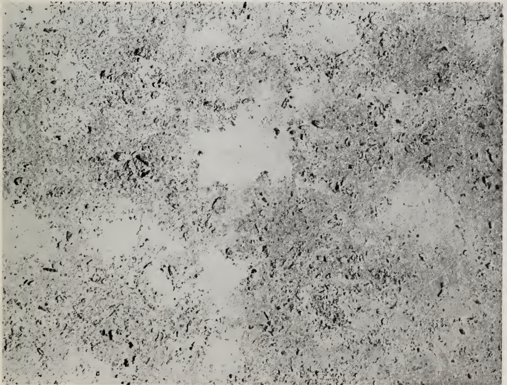
FIG. 4.—Travertine stone from the Niagaran dolomite. The dark spots are holes. Natural size.
