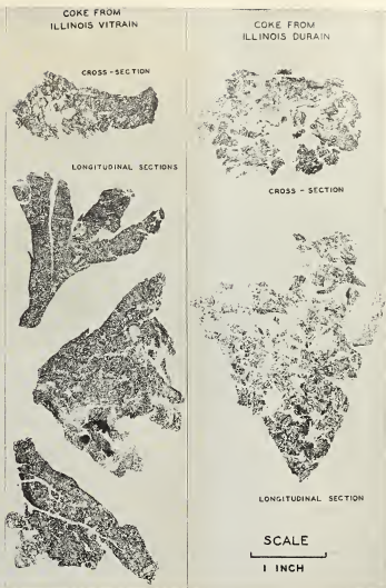
FIG. 3 SECTIONS OF COKE EMBEDDED IN PLASTER OF PARIS TO SHOW DIFFERENCES IN STRUCTURE
