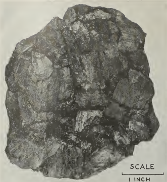
FIG. 4 FUSAIN AS IT OCCURS ON THE SURFACE OF A BLOCK (Breakage readily occurs at such surfaces and the broken fusain concentrates in the form of 100- to 200-mesh dust.)
