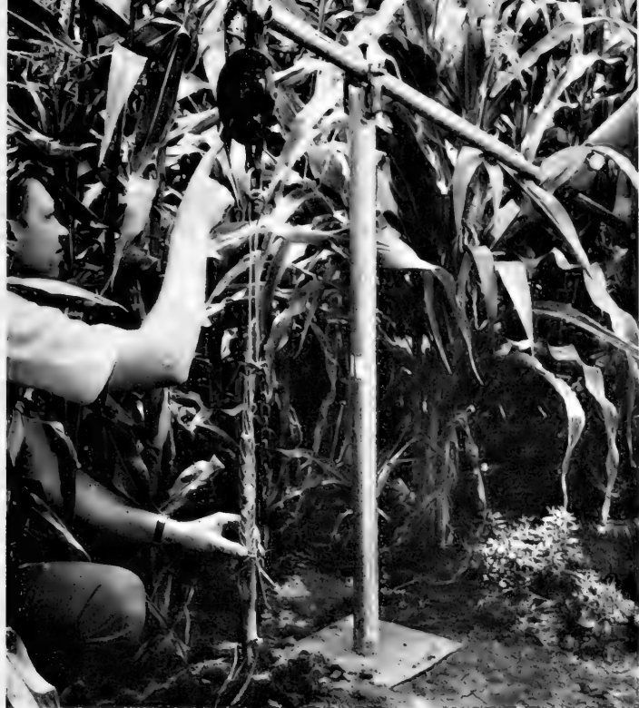
Vertical corn puller at work with Mr. Kuhlman pointing to gauge. (Photo by Survey photographer Wilmer Zehr.)
