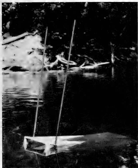
One of the sampling nets showing the top of its 1-foot square opening and the poles by which it is held in place in the river. At each station one net was placed near the bottom of the stream, a second at the top and just protruding, in order to catch anything floating on the surface. (Photo by Paul Fishman.)
