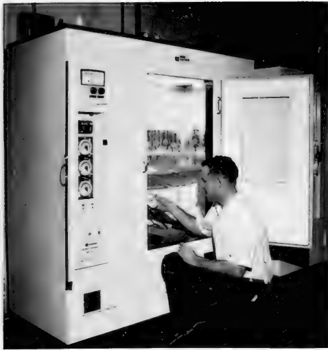
Cabinet-type growth chamber in which alfalfa weevils are reared continuously, independent of outdoor season. Settings for desired temperature, humidity, and light cycle and intensity are made on the control panel to the left. Dr. Armbrust is examining a dish of weevil eggs to record hatching. (Photo by Survey Photographer Wilmer Zehr.)
