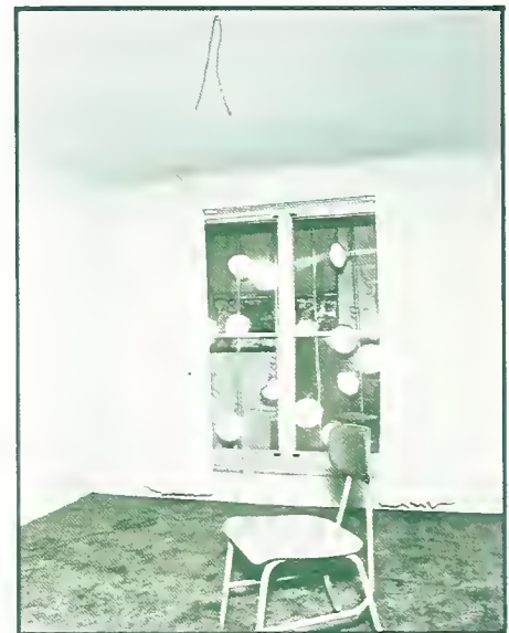
Inside the test room, one of four temperature and humidity probes can be seen hanging from the ceiling. Location of the other three probes is indicated in the diagram below.
