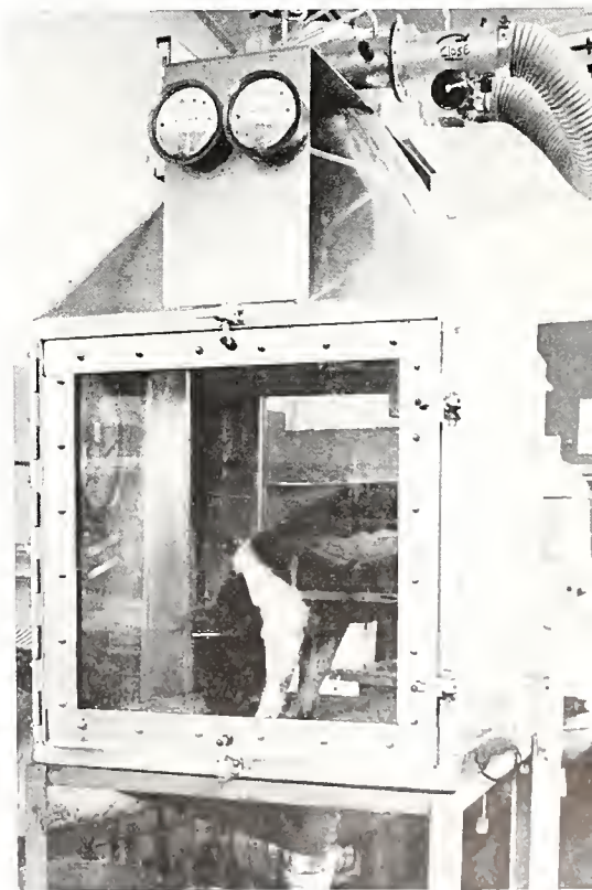
Pigs in this special chamber are exposed to a bacteria-containing mist. (Fig. 2)
