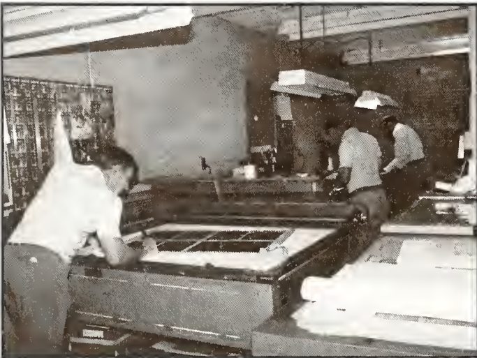
Negatives from the photographs are then stripped into their proper positions to make a "flat." In a final step, offset plates are made from the flats.
