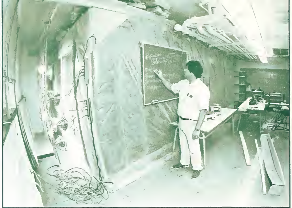
Author Mike Sherman is pictured in his laboratory, which houses the test room. This view, taken with a fisheye wide-angle lens, shows one of the insulated walls, the windows, and the external bank of lights.
