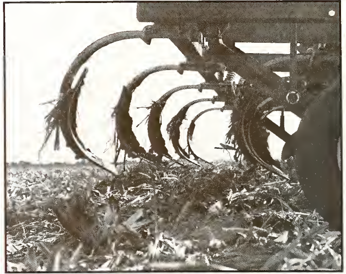
The business end of a chisel plow leaves crop residues on the roughened soil surface, thereby helping to reduce erosion.
