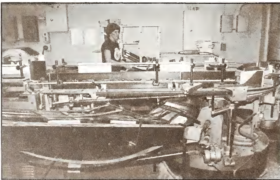
After printing, the signatures are sent to the bindery, where they are folded, assembled, trimmed, and bound. The machine pictured here assembles perfect-bound books.
