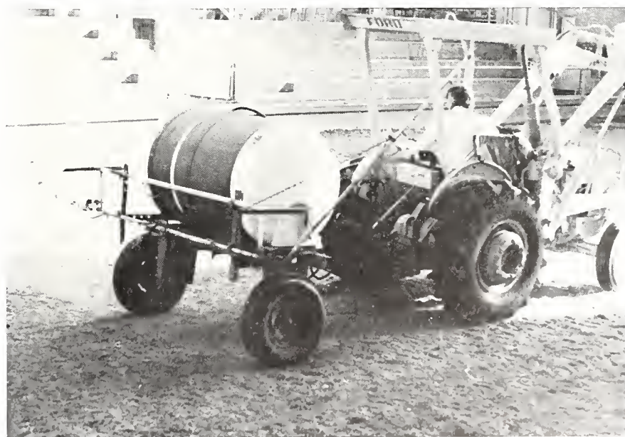
Fire-retardant solutions were applied by a power sprayer equipped with a 300-gallon tank and two side booms. Thirteen nozzles were spaced 20 inches apart, with each one delivering 0.35 gallon per minute at 30 pounds per square inch. (Fig. 2)
