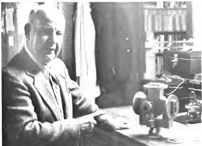
Electrical engineering professor Paul Coleman displays what he terms a vest pocket microwave accelerator and what textbooks designate as a ribatron. Developed by Coleman in 1946, the ribatron can generate up to 2,000,000 volts—a still unmatched record. (photo by Jay Zeff)
