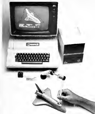
The Space Tablet allows the user to easily record coordinates by interfacing with an IBM or Apple computer.
