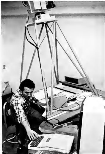
Todd Barrowclift, senior in biomechanics, employs an overhead single frame projector and computer located in the Biomechanics Research Laboratory. He is analyzing how gait patterns change in walking with no shoes to tennis shoes to high heels.
