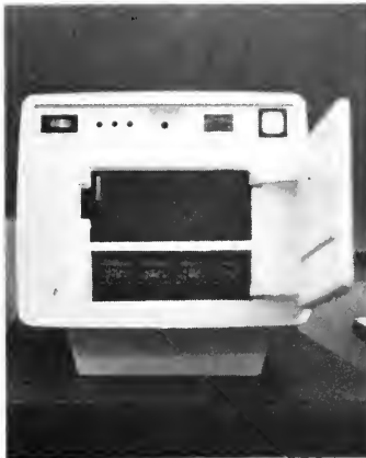
The VFR 2000 has the capability of transmitting the screen image to slide film in a matter of seconds (photo by Dave Colburn).
