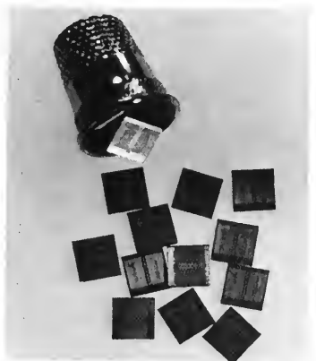
IBM's latest development is a 6.6 mm square, 32K bit static RAM chip with a read access time of 3 ns. At that speed, the entire contents of a 75 volume encyclopedia could be read in one second.
