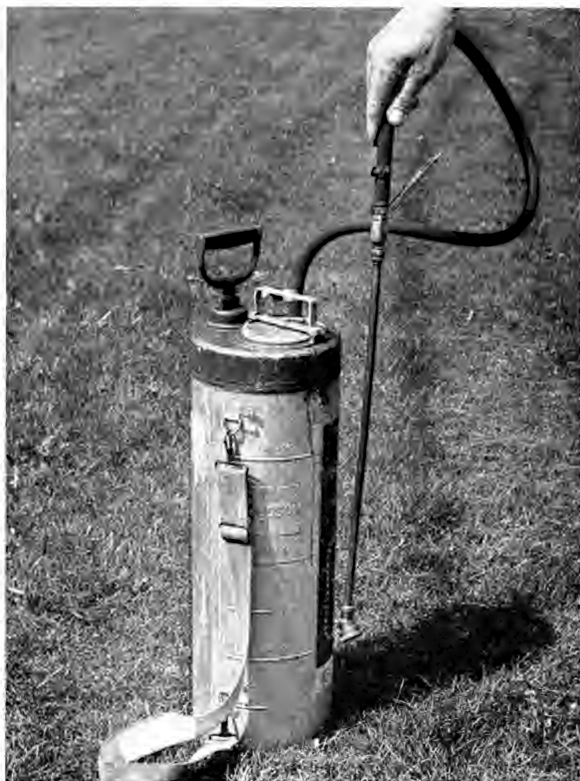
Fig. 55.—Compressed air sprayer, a convenient sprayer for small jobs.
