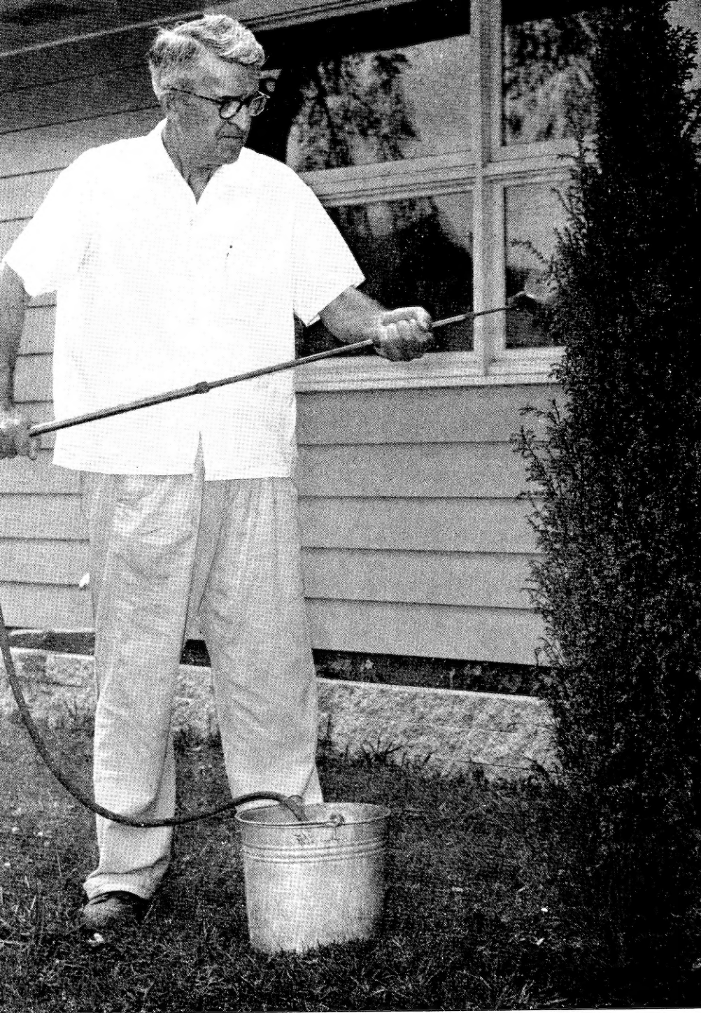
Trombone-type sprayer in use. This is an inexpensive sprayer that is convenient for applying chemicals to limited numbers of shrubs and small trees.
