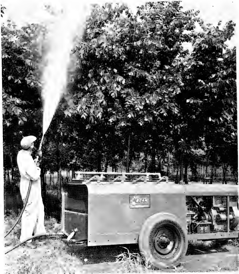
Fig. 58.—Power sprayer in operation. This machine, known as a hydraulic sprayer, will do an excellent job of spraying trees of small and medium sizes.
