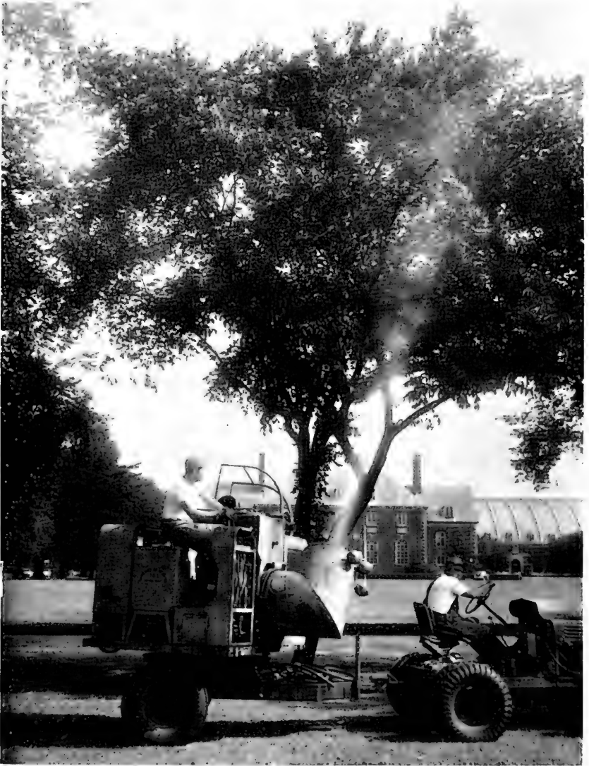
Fig. 59.—Mist blower or roto-mist sprayer in operation. This machine is particularly useful for spraying large trees.
