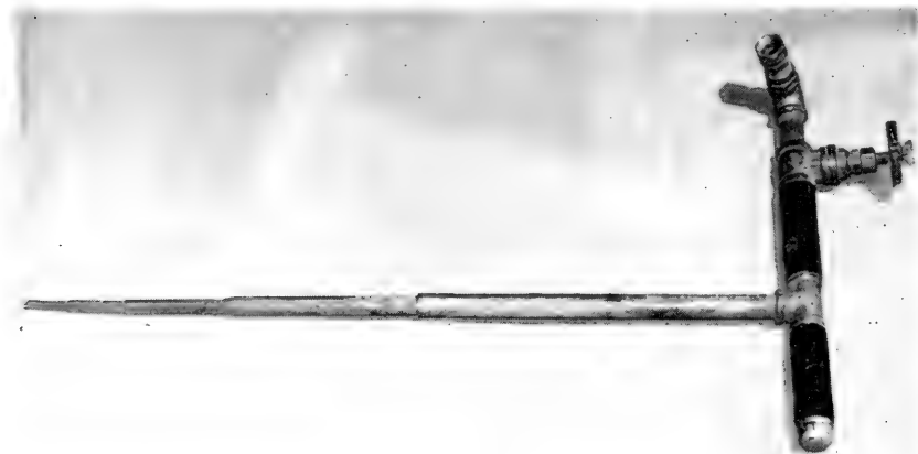
Fig. 33.—Feeding guns or lances can be devised by an ingenious individual who wishes to apply liquid plant food to his trees. Several types of these devices are manufactured and can be purchased.
