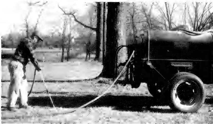
Fig. 32.—Hydraulic sprayers which develop several hundred pounds pressure can be used in liquid feeding of trees.
