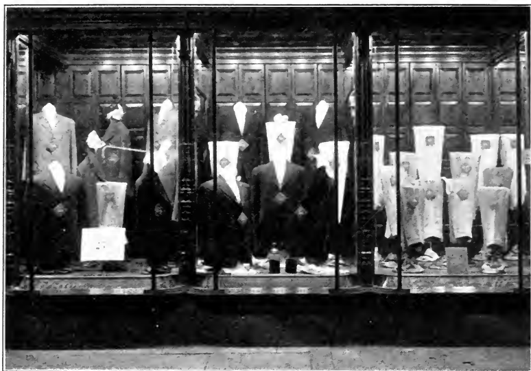
Fig. 19.—Show window in which the arrangement of lamps and reflectors was carefully calculated. The average intensity in this window was 30 foot-candles.
