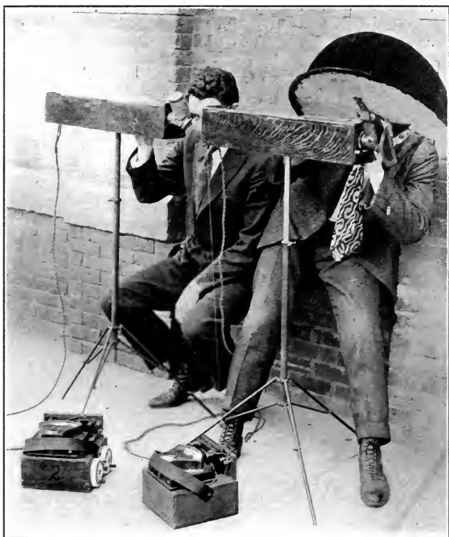
Fig. 18.—Simultaneous measurements with two photometers in determining daylight conditions.
