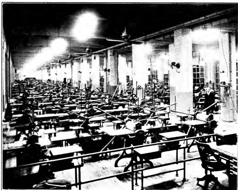
Fig. 6.—Hand press room in bureau of engraving and printing showing use of mercury vapor lamps.
