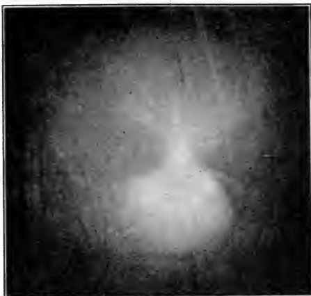
Fig. 9.—Screen illuminated at 10 ft. by parabolic reflector with star frosted "lens."
