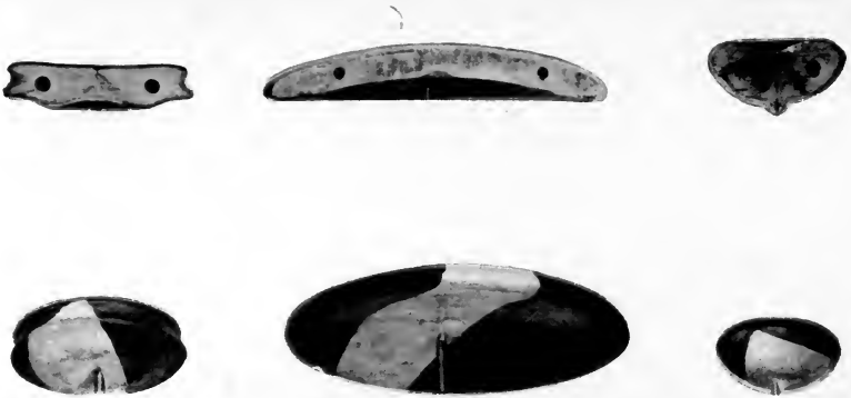
Fig. 7.—Solids representing distribution of candle-power corresponding respectively with Figs. 4, 5, and 6.
