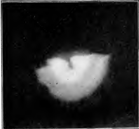
Fig. 11.—Screen illuminated at 10 ft. by paraboloid - ellipsoidal reflector with clear glass cover.
