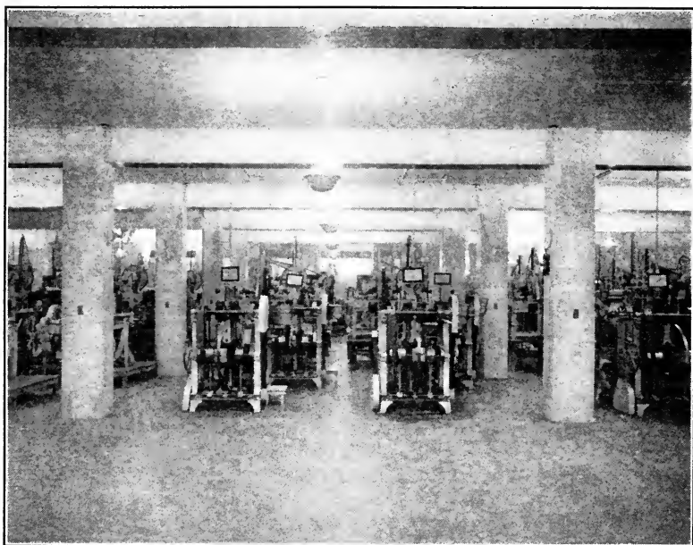
Fig. 3.—System of industrial indirect lighting with tungsten lamps.
