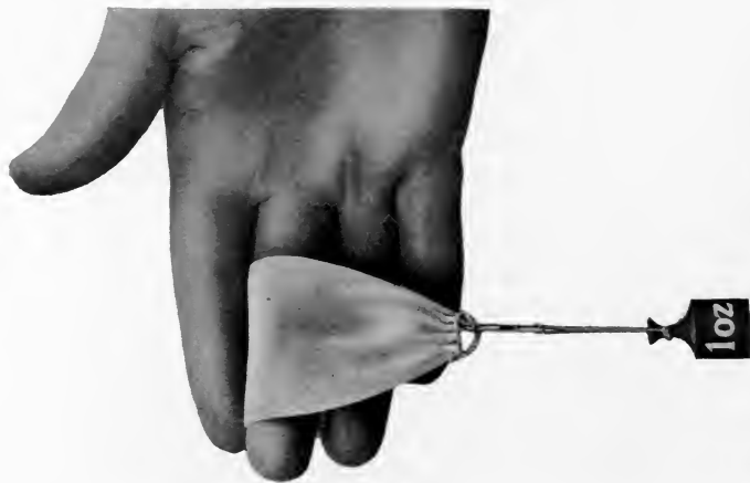
Fig. 1.—Demonstrating tensile strength of artificial silk mantle after burning .
