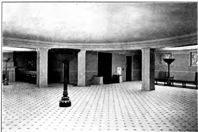
Fig. 29.—Indirect illumination of church lobby by means of floor standards.
