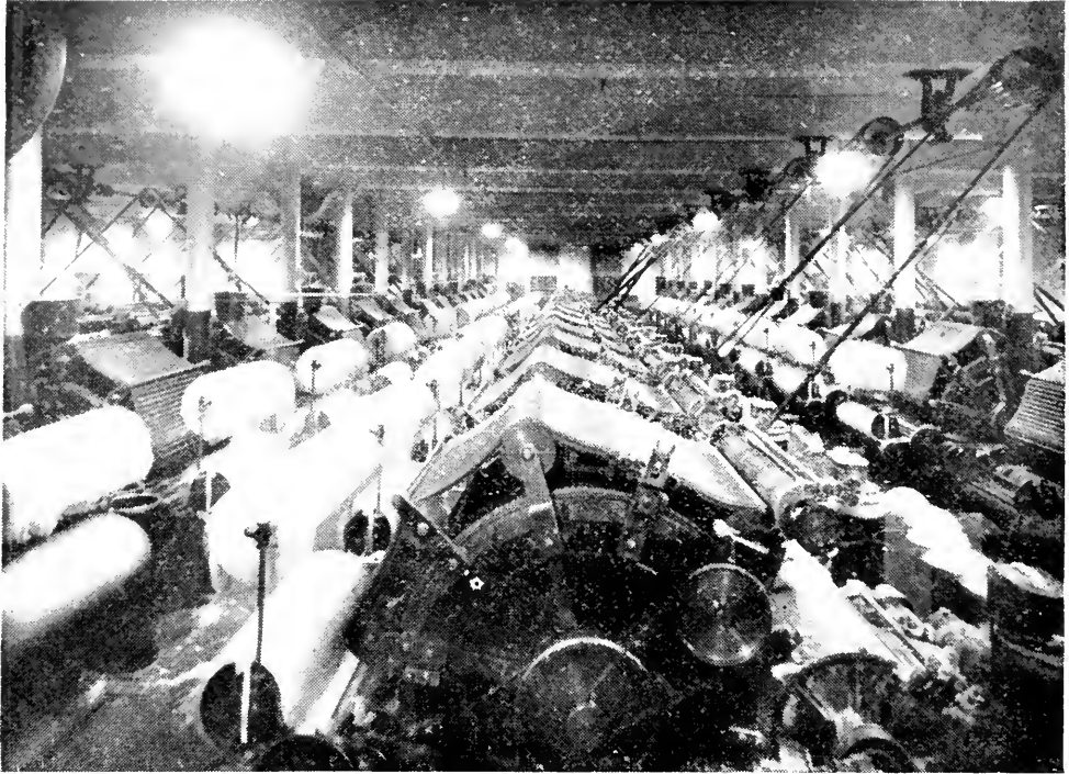
Fig. 3.—A card room with plenty of light in all work-aisles and between the machines, furnished by 150-watt bowl-enameled lamps on a spacing similar to that shown in Fig. 10.
