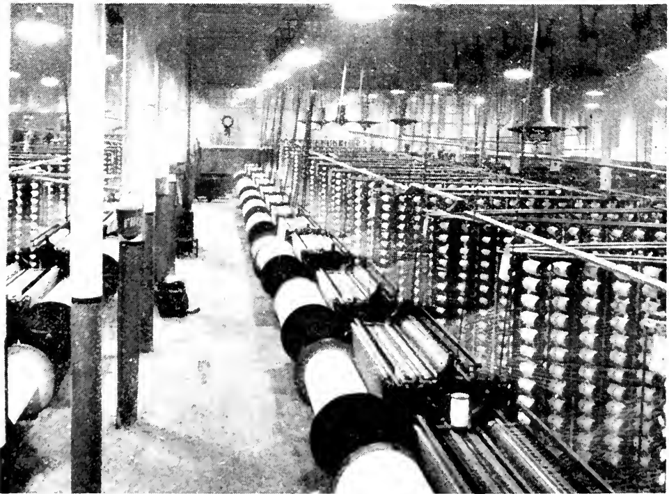
Fig. 4.—Warping requires a high level of well diffused illumination both at the beam and the creel. One hundred and fifty-watt units are spaced according to the suggestions of Fig. 16.
