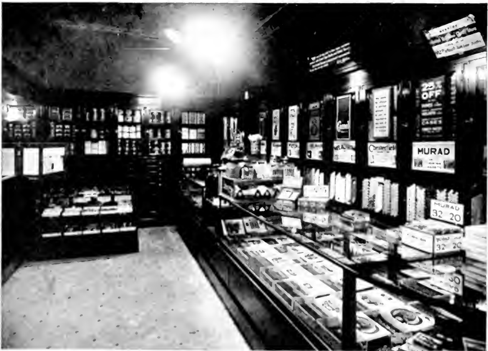
Fig. 5.—Night view of a typical cigar store (25 x 12 feet) illuminated by three 150 watt bowl frosted Mazda C lamps in prismatic glass deep bowl reflectors. Average intensity of illumination is approximately seven foot candles.
