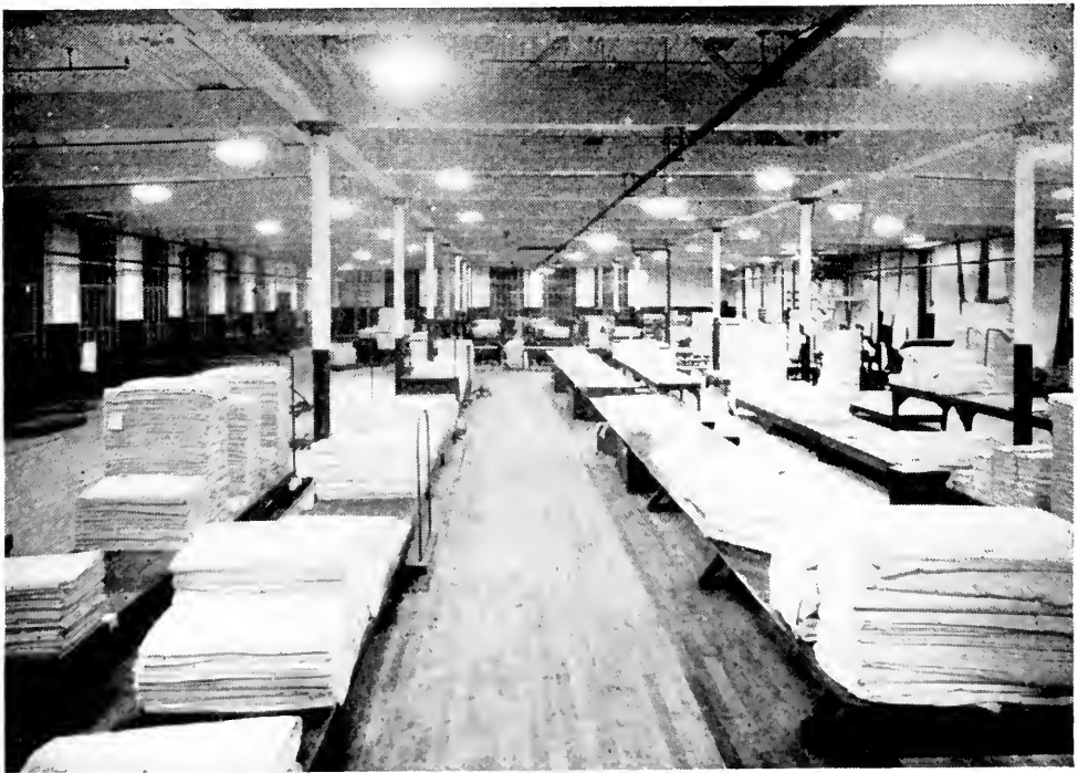
Fig. 20.—A well lighted cloth room. Two hundred watt diffusing units are spaced to obtain an illumination of 8 foot-candles.
