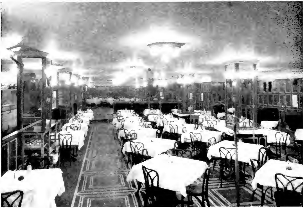
Fig. 2.— Cafeteria which illustrates the distressing effect of glare from the lighting system.
