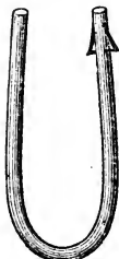
Fig. 66.—Catch for Ox-Bow. and secures it as soon as it reaches the notch.
