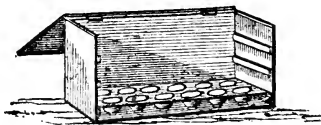
Fig. 9.—Section of chest for carrying earthen bowls of fruit—showing board with holes to receive them.
