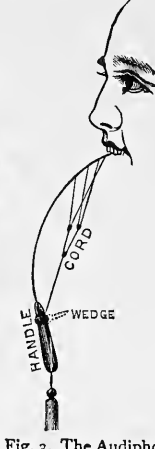
Fig. 3. The Audiphone properly adjusted to the upper teeth; ready for use. (Side view.)
