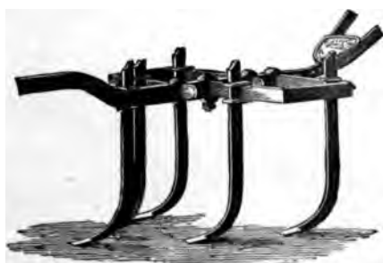
Representing the 5-tined Scuffler or Stirrer, fitted in same frame in lieu of Hoes.
