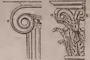
Volutes of the Ionic and Corinthian Capitals a a , Volutes. b , Helix.
