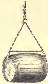
Sling used in unloading Vessels.
