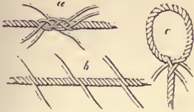
Splices of Ropes. a, Short Splice. b, Long Splice. c, Eye Splice.
