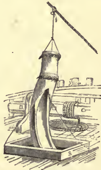
Wind-sail suspended from jib-stay.
