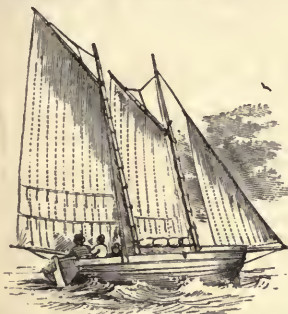
A wherry with fore-sail reefed, the main-sail showing reef-bands and reef-ties.
