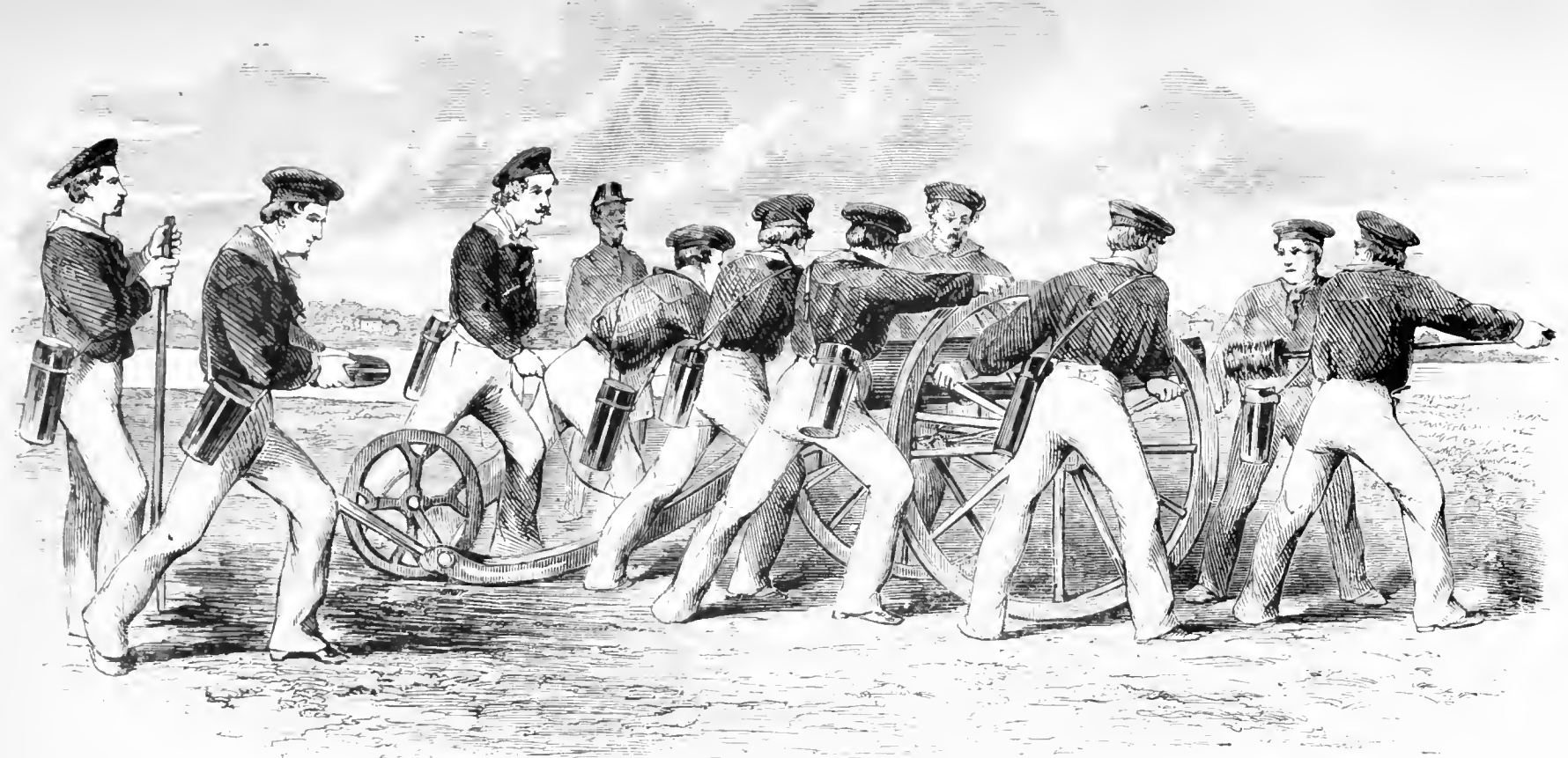
LAND PRACTICE OF SAILORS WITH THE DAHLGREN HOWITZER BOAT GUN—SPONGING OUT THE GUN.
