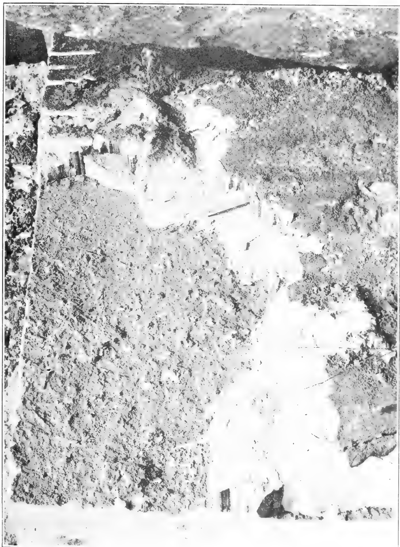
FIG. 5.—Block of Salem limestone split along a large stylolite-seam. Note the slickensided side-surfaces of the exposed columns (marked by the ruler).
