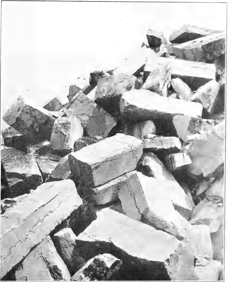
FIG. 18.—Pile of waste stone, a result, for the most part, of stylolite-seams. The Consolidated Stone Company, Dark Hollow district, Lawrence County, Ind.
