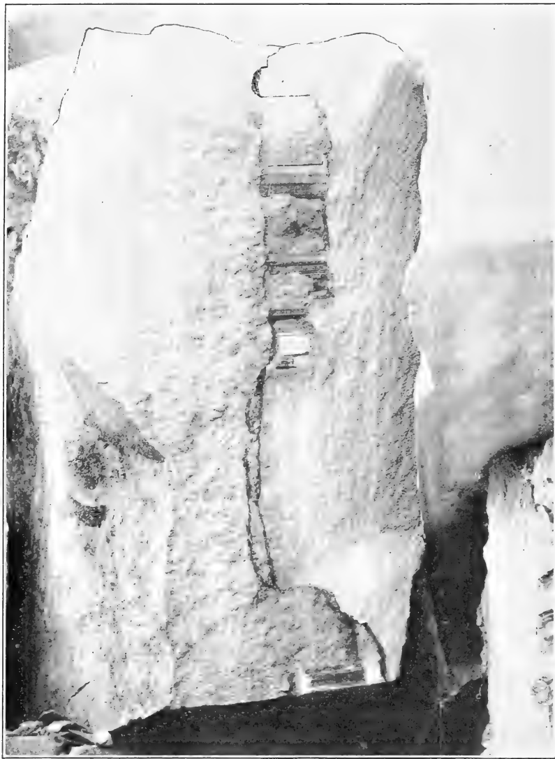
FIG. 34.—Stylolites of the Salem limestone, showing a double clay parting, separated by a thin layer of limestone, at the top of the wide column on the left. The other columns have single clay caps. Note the well-defined striations on the sides of the columns at the right. From a quarry of the Consolidated Stone Company, Dark Hollow district, Lawrence County, Ind.
