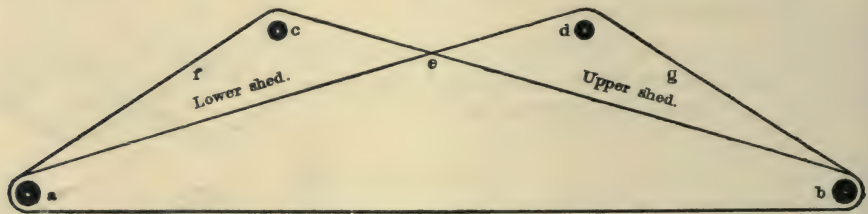
FIG. 188.—Diagram showing formation of warp of sash
