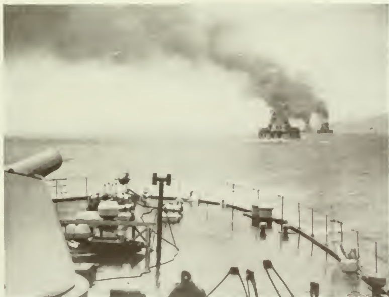
The above photograph as published. Smoke was added to obscure the fire-control of the ships
