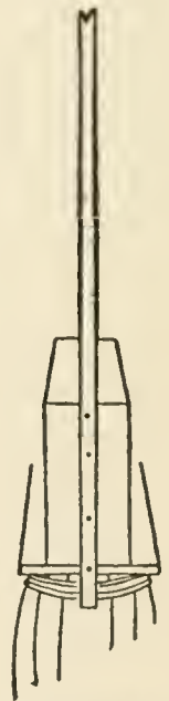
Fig. 521.—Nail upright on box and end of board this way.
