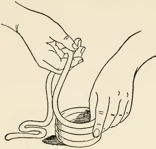
Fig. 325.—Lift the roll and build up the sides.
